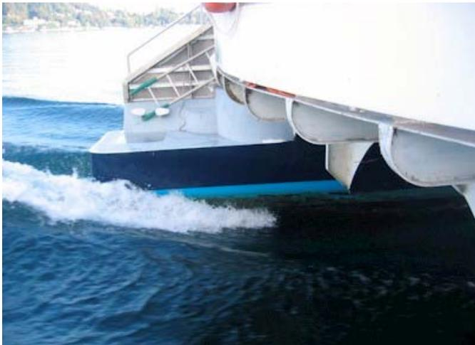
At 2000 RPM, approximately 12 knots, on the inside between the hulls the flat part of the stern is almost completely out of the water. Only about 1 meter touches the water. On the picture this point is where the white spray starts.
