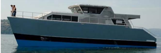
As can be seen from the picture, the cat is very light up front, but the whole anchoring equipment is missing up front.
