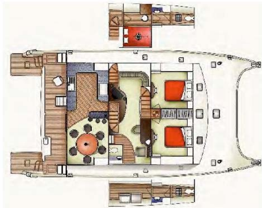
The layout of Malcolm Tennant's New Yorker. The heads are not really luxurious (where are the bidets?) and the third cabin under the bridge must be rather claustrophobic.
