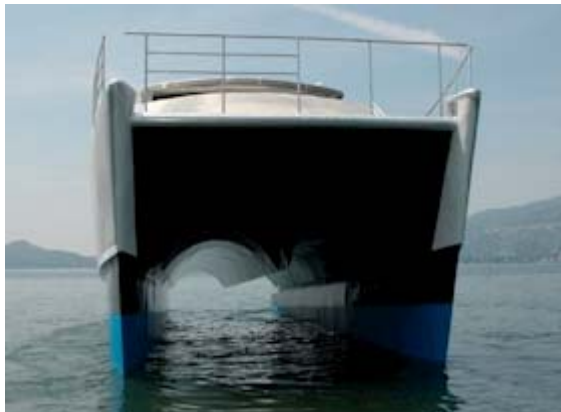
The front view of the PH8. You cannot lower the anti-slam nacelle (the middle keel, above the water level), without compromising bad whether capability.
