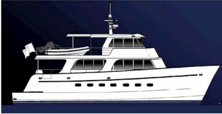
A 21 m "expeditionary" catamaran designed by Malcolm Tennant. To gain space the pilothouse is placed above the cabins.
